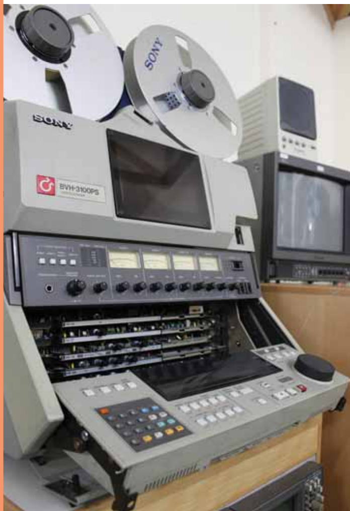
Sony BVH-3100PS. 1-inch VT open reel video recorder
