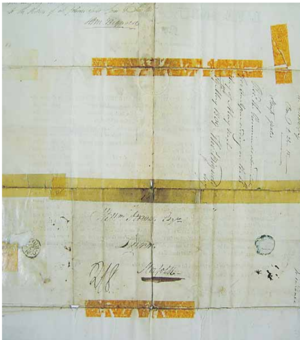
Verso of document showing moisture sensitive tape and pressure sensitive tape
