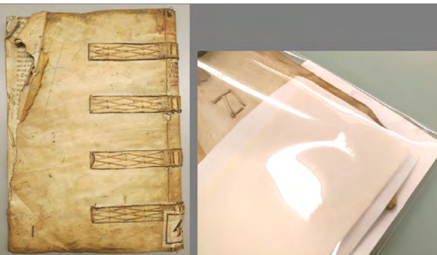
Humidification of parchment with Gore-tex, Tekwipe and Mylar L-sleeves. Acknowledgement: K.Beaty, Harvard Business Medici Collection.
