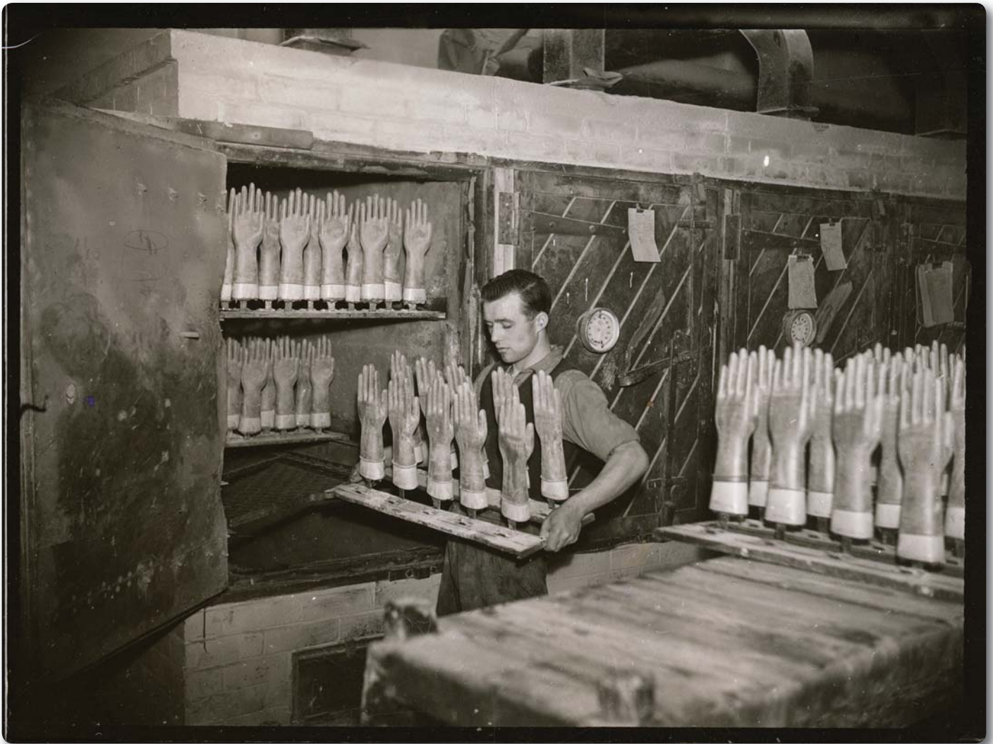
A man placing rubber gloves on moulds into an oven in a factory producing rubber gloves. 20th January 1939. Photograph courtesy of Historic England Archive
