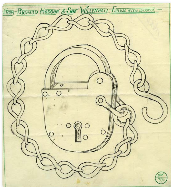
A hand drawn 1911 design for a Hodson lighter lock manufactured primarily for the London market (WHLLMA/A/1/613, Locksmith's House Archive Collection), courtesy of the Black Country Living Museum
