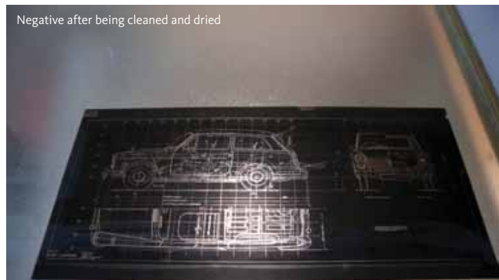
Test using cross polarized filters to confirm polyester base
